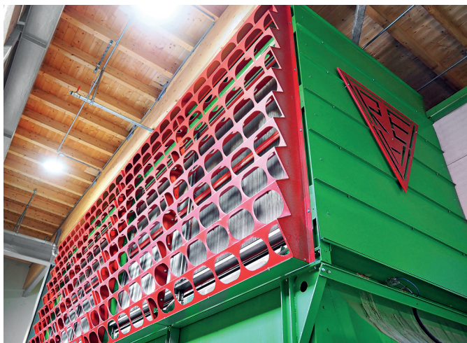
To ensure the efficient operation of the belt dryer, Rudnick & Enners installed a belt dryer with an integrated heat unit
