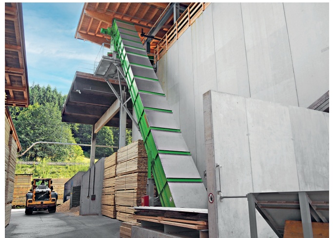
A wheel loader feeds the sawdust into a specially designed infeed station. Then, the sawdust is buffered inside a 1,000-stere rectangular container
